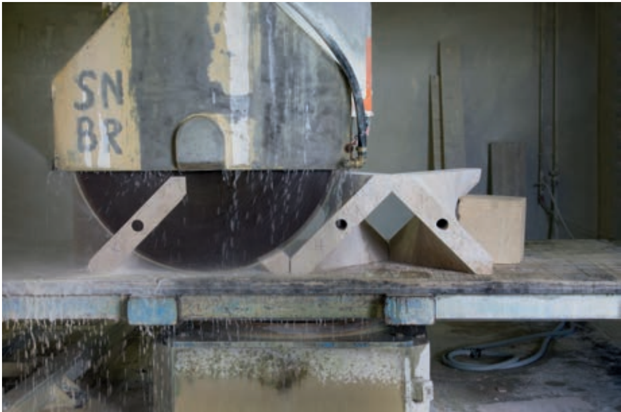
Fabrication of a french limestone vault prototype that produces almost no material waste, 2017. Architects: New Fundamentals Research Group. CNC fabrication: SNBR, Troyes, France.
